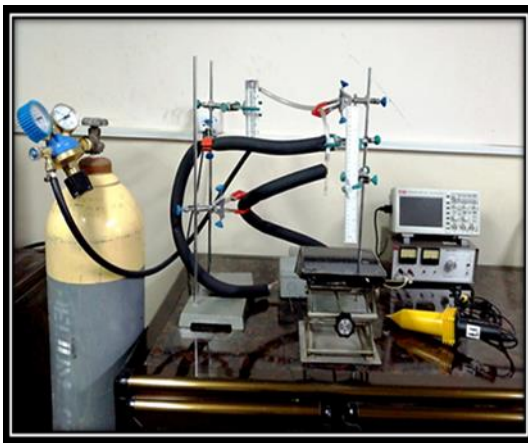
Fig. 1. The plasma system that was designed by the researcher [12] (a picture inside the scientific laboratory, diagram)
